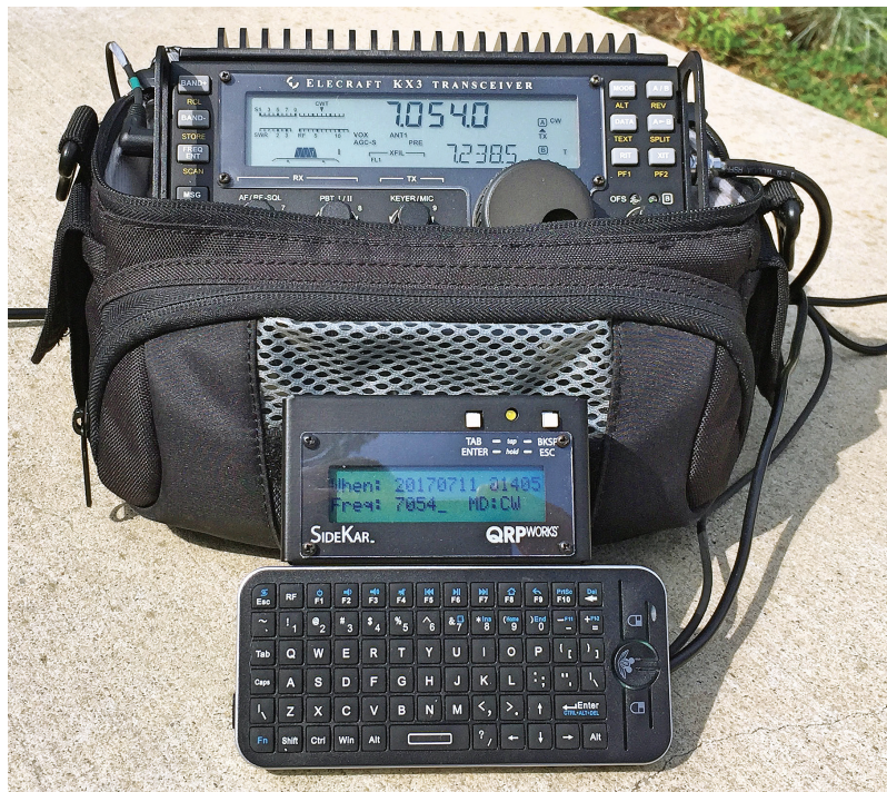
Figure 21 — The SideKar and compact wireless keyboard with the author's KX3 transceiver.
