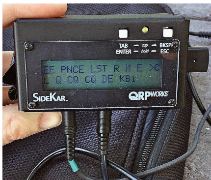
Figure 22 — Transmitted text rolling across the SideKar screen.
