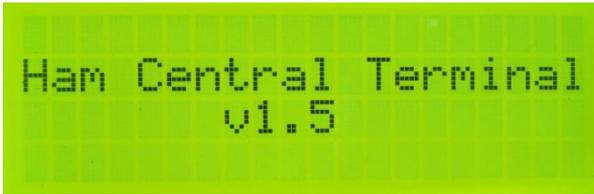
The HCT will then automatically attempt to connect with the rig via its serial port. It will try every rig baud rate possible (starting with the fastest) until it establishes a connection. And it will retry a number of times before giving up. During the retries, the HCT screen will show a series of progression dots. Each dot is a try at each of the four baud rates (38400, 19200, 9600, and 4800).
