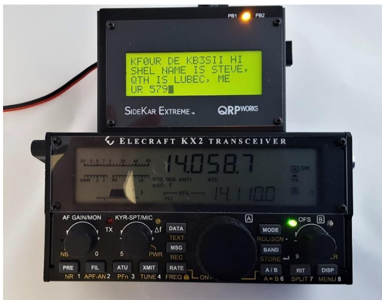
SideKar Extreme shown installed, but the SideKar Decoder Edition is installed the same way.
