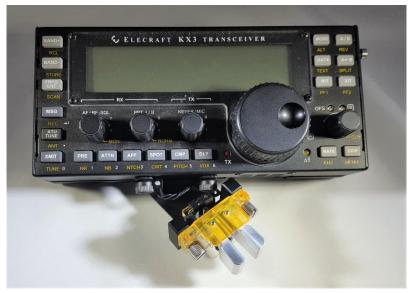
Note: If the cable is removed from the Key Line Pi, note that when reinstalling it onto the right-angle pin extender, the gold dot faces up.
