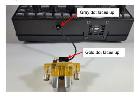
4. Attached the Key Line Pi bracket to the rig in place of the paddle. Hand tighten the two Key Line Pi thumbscrews. Swivel the bracket as necessary to reach the thumbscrews.
