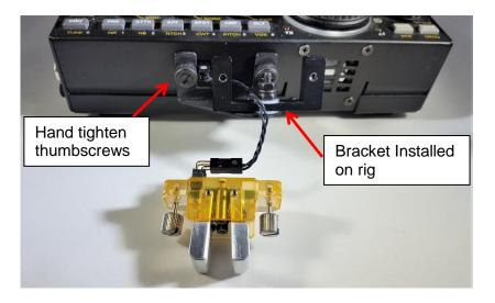
5. Attached the paddle to the Key Line Pi by hand tightening the two
