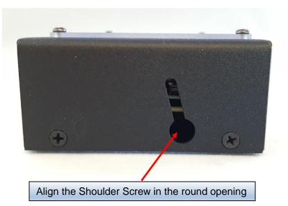
Slide / wiggle the SideKar Extreme down until the notch at the bottom of the SideKar Extreme bracket is under the KX3's thumbscrew head. If the SideKar Extreme hits the BNC connector, the bracket is installed backwards. Remove it and put the longer slot against the SideKar Extreme.
