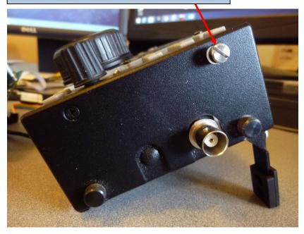
3. Loosen, but do not remove, the thumbscrew for the KX3 right foot. Fold the KX3 foot under the KX3 so it is not extended.
