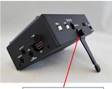
Flat head screw removed. Tall leg installed with a thumbscrew.
