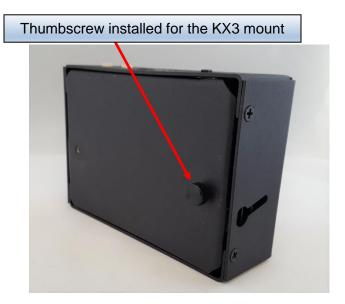
5. Install the KX3 mounting bracket under the thumbscrew as shown. Tighten the thumbscrew so the bracket is snug. The bracket edge should be even with the side of the SideKar Extreme.
