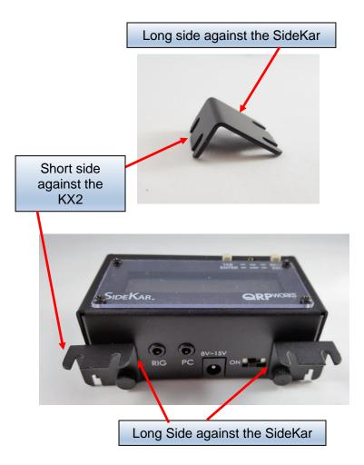
3. Slide the 2 brackets on the SideKar under the thumbscrews on the back of the KX2. Tighten the thumbscrews.
