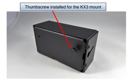
5. Install the KX3 mounting bracket under the thumbscrew as shown. Tighten the thumbscrew so the bracket is snug. The bracket edge should be even with the side of the SideKar.
