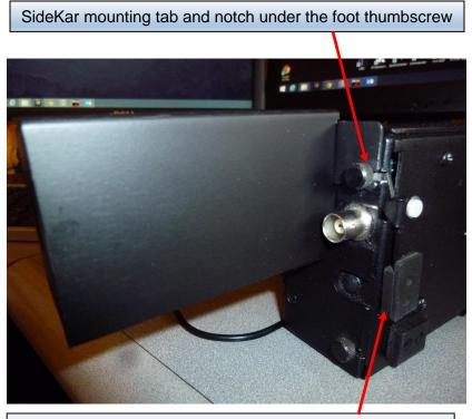
Extend the foot after lightly tightening the thumbscrew
