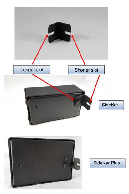
6. Position the SideKar so the installed shoulder screw on the KX3 is in the round portion of the keyed slot and flat against the KX3.
