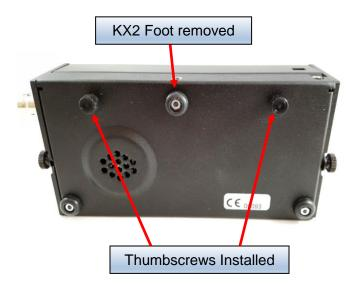
2. If not already installed, install 2 supplied thumbscrews in the bottom 2 holes in the SideKar. (lower right of the On-Off switch, and lower left of the Rig port.) Install the 2 KX2 brackets under the thumbscrews as shown.
