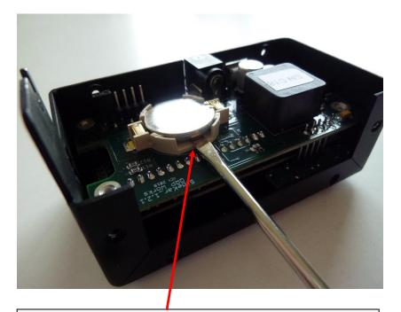
Remove the battery by inserting a small flat blade screwdriver between the bottom of the battery and the battery holder as shown. Twist the screwdriver between the battery and the holder to pop the battery out. Do **NOT** lift or pull the battery up. It might pull the battery holder off of the PC board. Hold the battery holder down while twisting the screwdriver to be sure.
