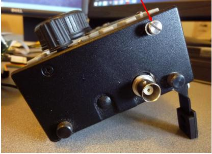
Loosen, but do not remove, the thumbscrew for the KX3 right foot. Fold the KX3 foot under the KX3 so it is not extended.
