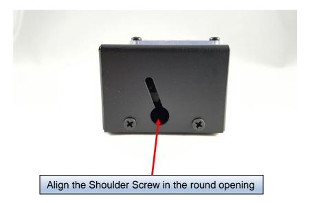
Slide / wiggle the SideKar down until the notch at the bottom of the SideKar bracket is under the KX3's thumbscrew head. If the SideKar hits the BNC connector, the bracket is installed backwards. Remove it and put the longer slot against the SideKar.
